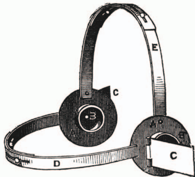
Fig 8. Left—“Pseudoscopic Thompson” by Nicholas Wade. Silvanus Phillips Thompson is shown with his left and right eyes superimposed. Right—his illustration of the pseudophone which he described in the following way: “The simple instrument for which the author suggests the name Pseudophone consists of a pair of ear-pieces, A A, furnished with adjustable metallic flaps or reflectors of sound, C C, which can be fitted to the ears by proper straps, D and E, and can be set at any desired angle with respect to the axis of the ears, and can also be turned upon a revolving collar about that axis so as to reflect sounds into the ears from any desired direction.” 52
